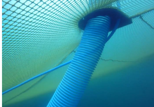
Figur 9. LiftUp slange under nottak under drift
