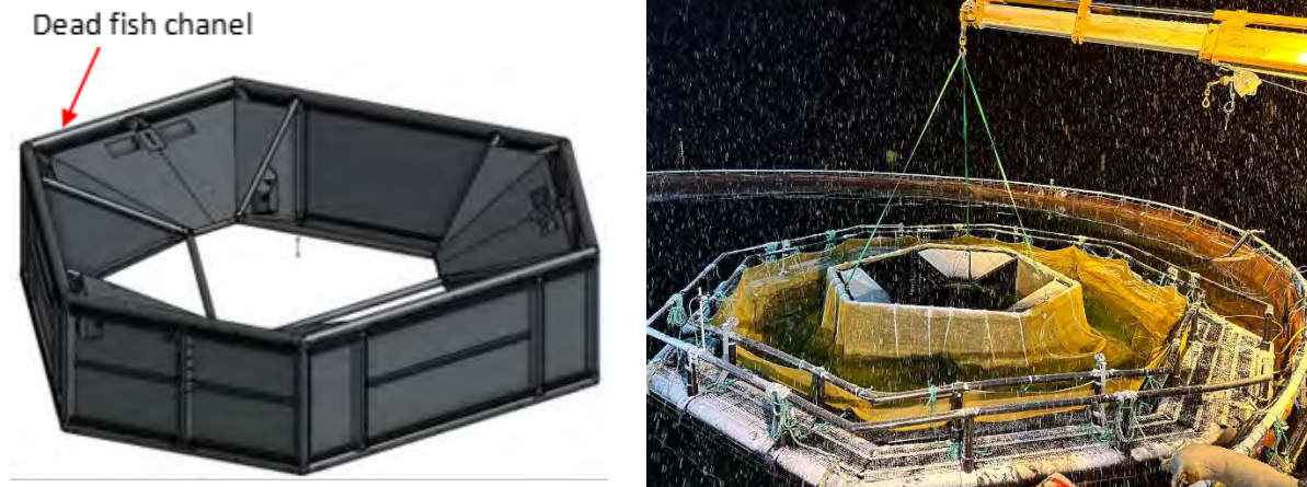
Figure 7 Technical specifications and information for the iFarm floater, snorkel, bottom ring and docking stations (Figure 5a, left) and a picture (Figure 5b, right) showing the installation of a docking station for Phase 3 in one of the iFarm cages. Note the inflated air tube at the base of the docking station.
