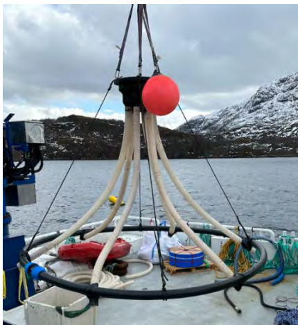
Figure 3c, iFarm subfeeder used in M10 with diameter 5 m
