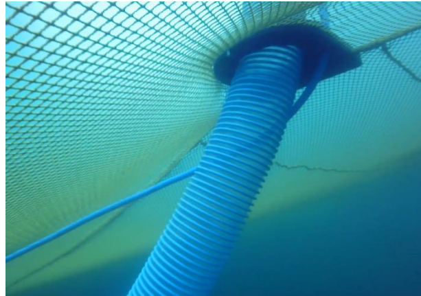
Figur 8. LiftUp slange under nottak under drift
