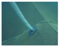
Figure 3b, Feed hose mounting in net roof
